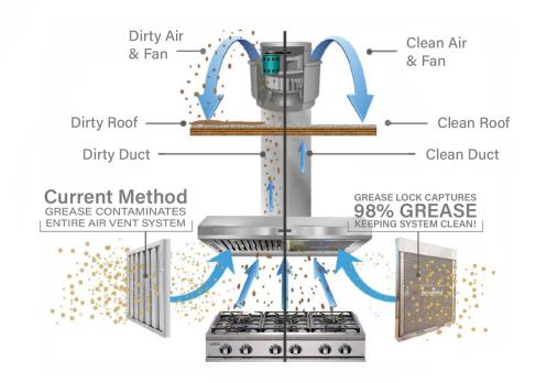
With The Grease Lock Filter System You Can:
